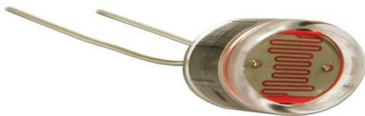
Fig. 6: Light Dependent Resistor or Sensor.
